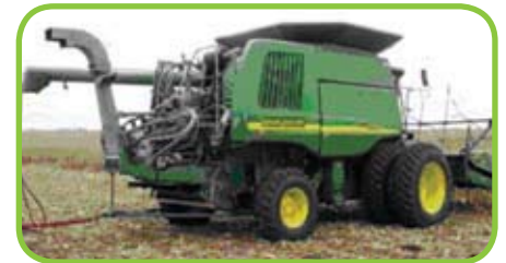
The single-pass harvester, which is being developed with DOE and USDA funding, enables farmers to harvest corn stover (stalks, cobs, and leaves) and grain with one pass through a field (Image courtesy of Iowa State University).
